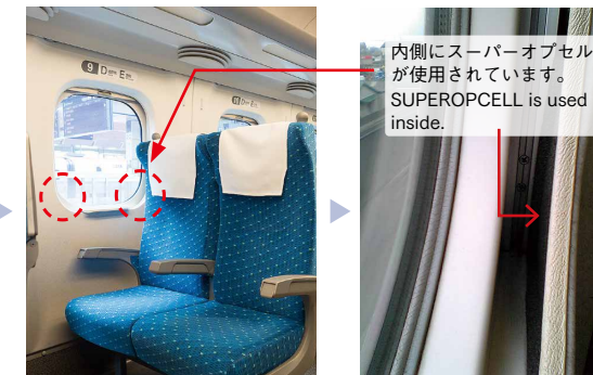
客室窓枠(吸音材・隙間埋め材(難燃性)) Passenger-car window frames [sound-absorbing material, material for filling clearances (fire-retarding)]
